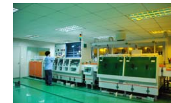
Developing and rinsing of soldermask
