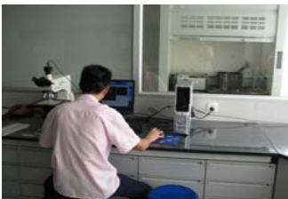
Physical Laboratory Cross sectioning preparation to check hole wall thickness and quality
